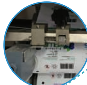
Web guide sensor with fine control knob
